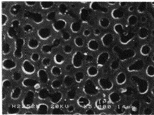
Fig.5. SEM of porous polyimide surface (PI/PU: 20/80, 350°C)
