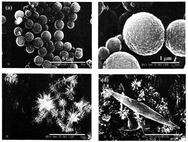
Figure 2. Morphology of PPPI. Micrographs of (a) and (b) are the microspheres of Run No. 1. Those of (c) and (d) are the star-like aggregates of needle crystals and the lozenge-shaped crystals of Run No. 7.
