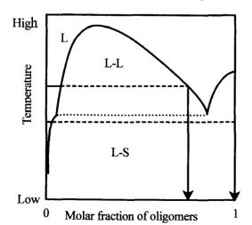
Scheme 2. Schematic C-T phase diagram for partially miscible oligomers and solvent system. L: miscible liquid phase, L-L: two immiscible liquid phase, L-S: liquid-and solid phase
