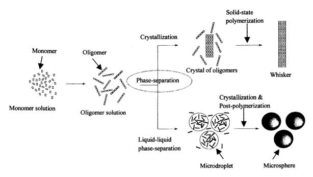
Scheme 1. Concept for morphology control by means of phase separation of oligomer during solution polymerization.
