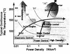
Fig. 4 Power density treds in car electronics
