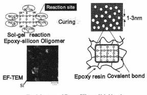
Fig. 8 Concept of Epoxy-Silicone Hybrid resin
