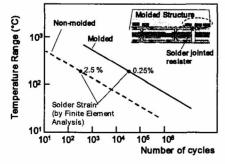
Fig. 6 Reliability of Solder Joints of Resister
