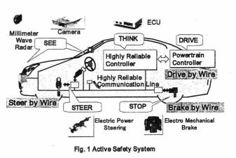
electric /electronic components of x-by-wire systems are required to be mounted in harsh environments such as on/in engines with high temperatures, high vibration and highly corrosive conditions which may damage the components.
