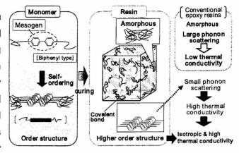
Fig. 10 Concept of Thermal Conductive
