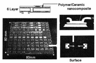
Fig. 15 6-layer Wiring substrate with embedded capaciter
