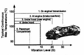
Fig. 3 Temerature and vibration level in various place of car
