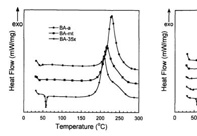
Fig. 1 DSC thermograms of three types of arylamine-based benzoxazine resins.
