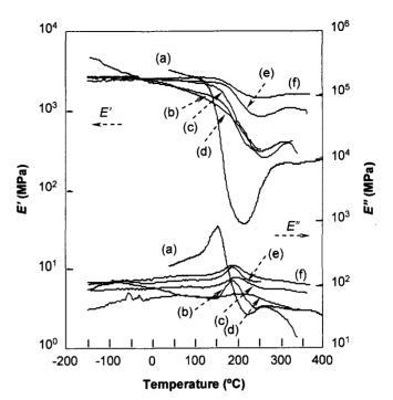
Figure 3. DMA results of pristine PBa (a), PBa-PDMS(20%) (b), PBa-PMPS(20%) (c), PBa-PMPS(40%) (d), PBa-PDPS(20%) (e) and PBa-PDPS(40%) (f) hybrid.
