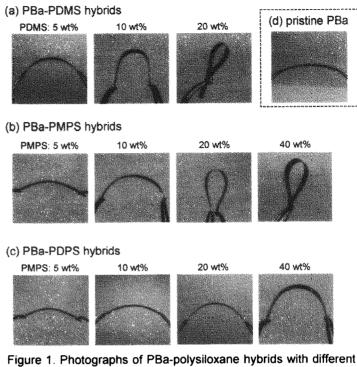
type of polysiloxane at various polysiloxane contents (a-c). The photograph of pristine PBa film is also shown in the dotted square (d). The size of bent film is 4 mm x 50 mm x ca. 200 mm.
