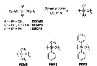
Scheme 2. Synthesis of polysiloxanes by sol-gel process.
