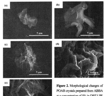
POAB crystals prepared from ABBA at a concentration of 5% in DBT-LPF at  $350^{\circ}$ C for (a) 10 min, (b) 30 min, (c, d) 1 h and (e) 2 h.
