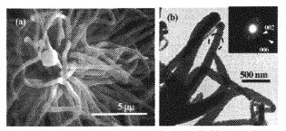
Figure 1 (a) SEM and (b) TEM of POAB fibrillar crystals
