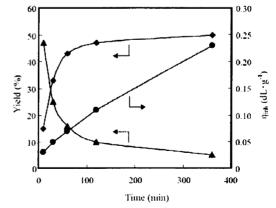
Figure 3. Plots of yield ( $\blacklozenge$ ) and inherent viscosity ( $\blacklozenge$ ) of POAB crystals and yield of oligomers recovered from filtrate ( $\blacktriangle$ ) as a function of polymerization time. Polymerizations were carried out from ABBA at a concentration of 5% in DBT-LPF at 350°C.
