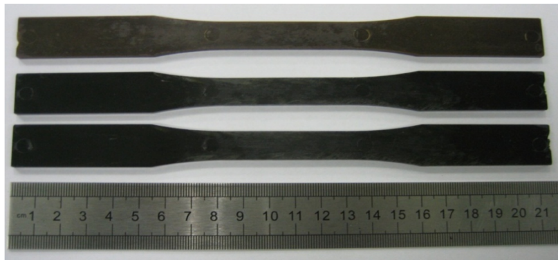
Fig1. Dumbbell-shaped test specimens of AURUM by injection molding
