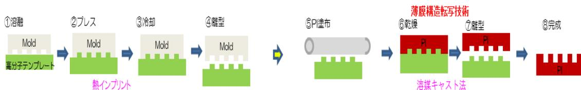
Fig.1 Fabrication process of Polymer film
