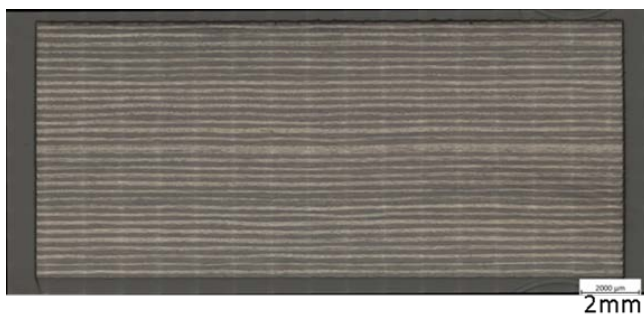
Fig. 3 Optical micrograph of TriA-X CFRP of 64 plies (t = 8.8 mm)
