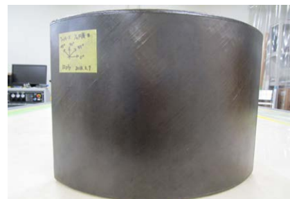
Fig. 4 1/4 Cylindrical structure of TriA-X CFRP (R 200 mm, L 210 mm, [-45/0/45/90] 2S )
